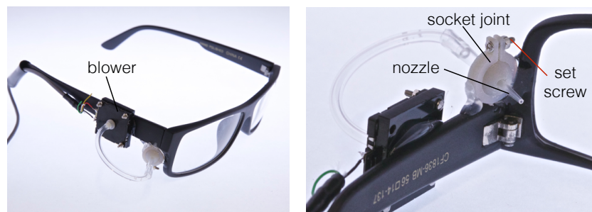
Fig. 6. Glasses with the air puff, that were used in the user study. A close up of the nozzle assembly is shown on the right.
