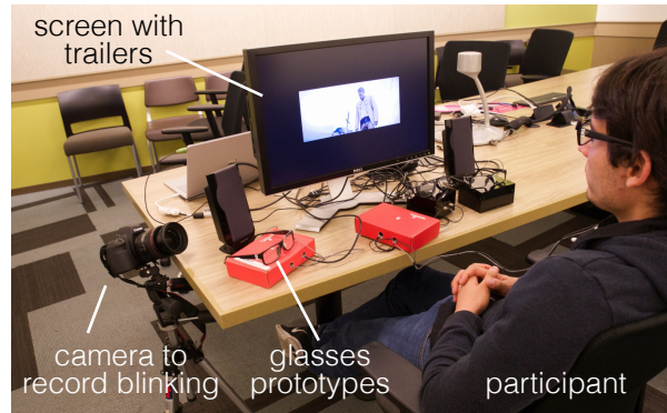
Fig. 7. The setup during the first and second setup. The participant watched trailers on the monitor while wearing each of the four prototype glasses.
